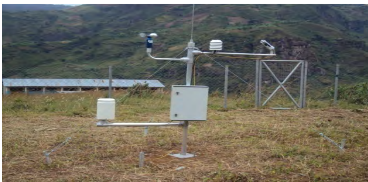
Plate 2: Hydro-meteorological equipment fixed for hydrological monitoring
