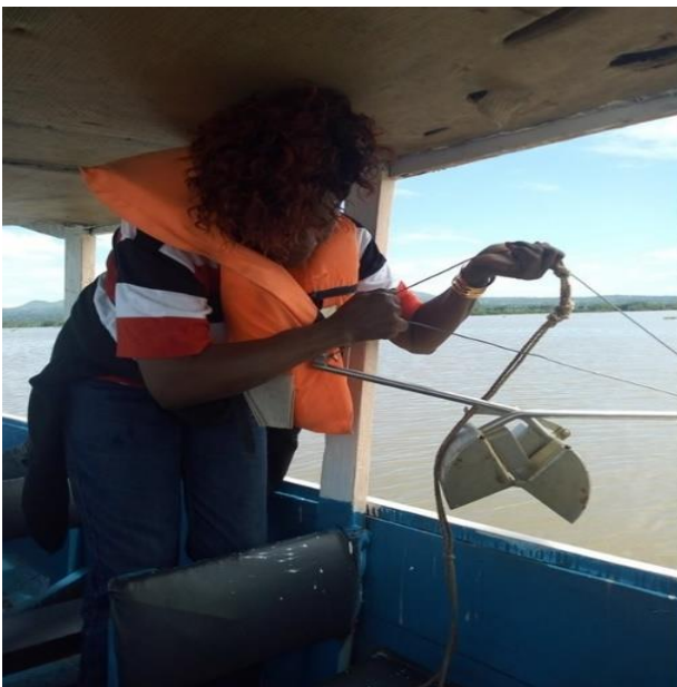
Ekman grab sampler for sediments
