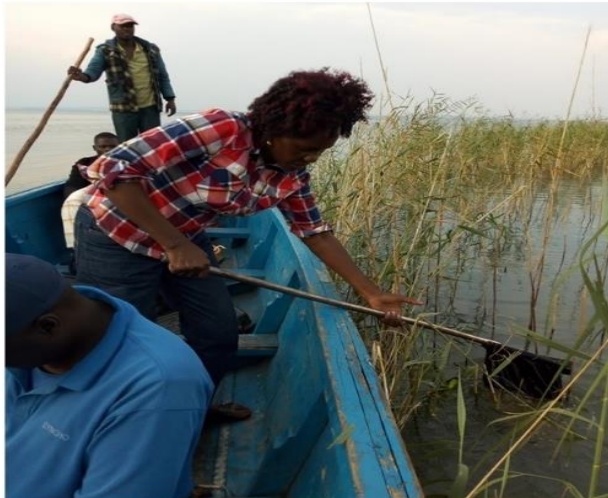
Scoopnet for shoreline sampling macro-invertebrates
