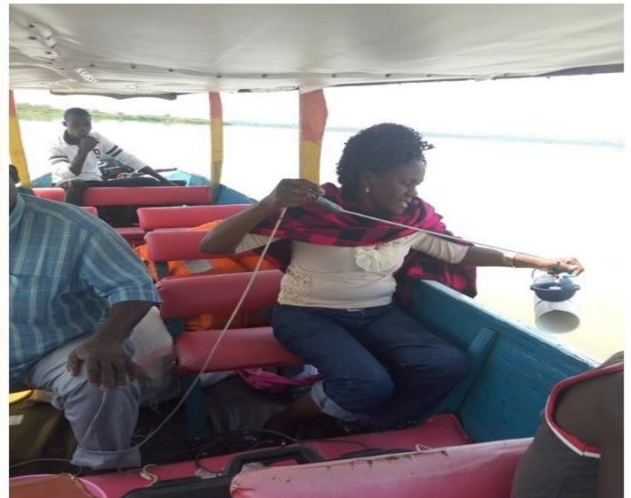
Vandon for sampling water
