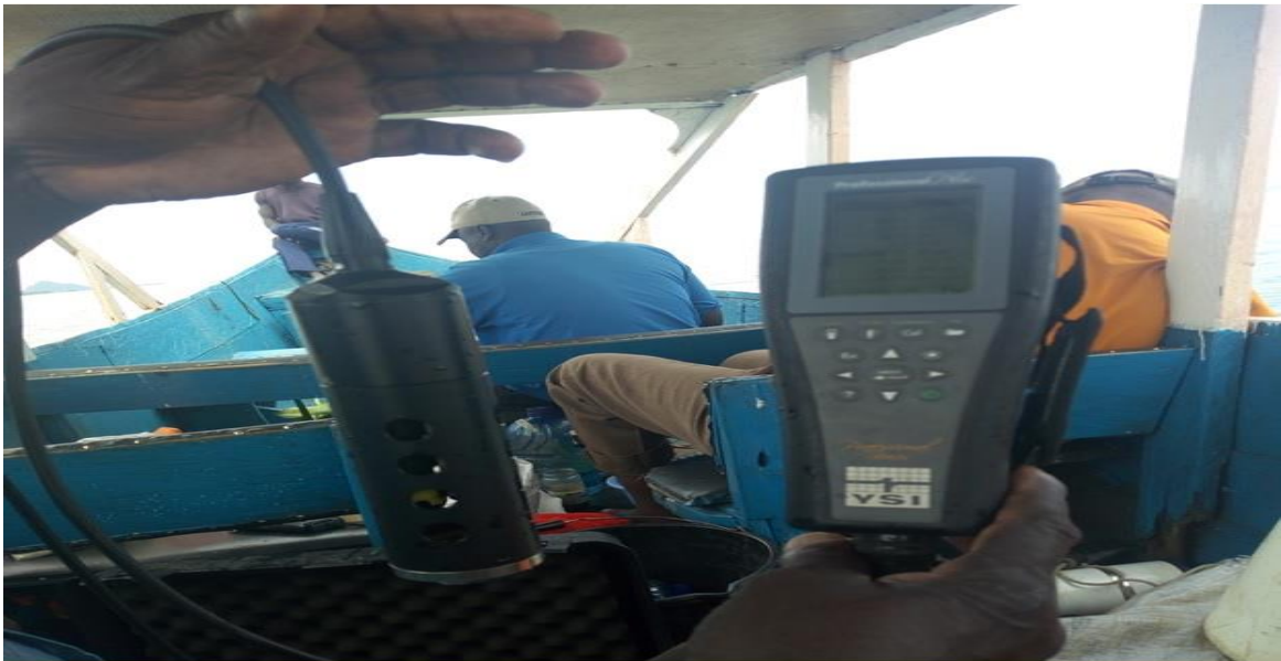
Figure 3.6: YSI meter for water Physico-Chemical parameters Source: Fieldwork photo
